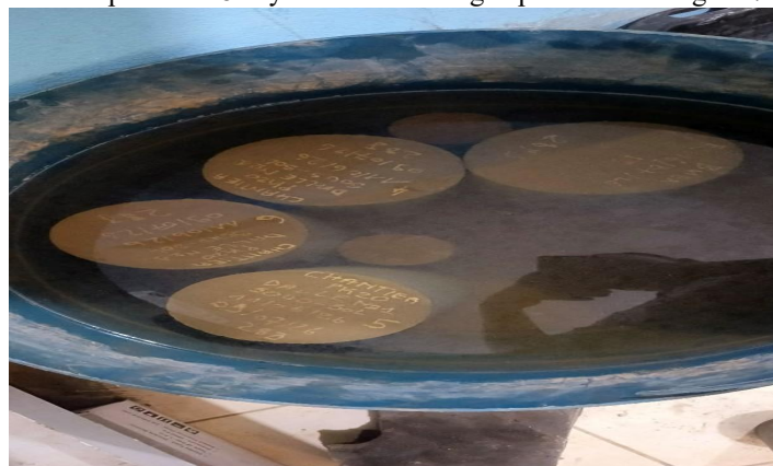
Figure 7: Immersion of test samples for 28 days before crushing
