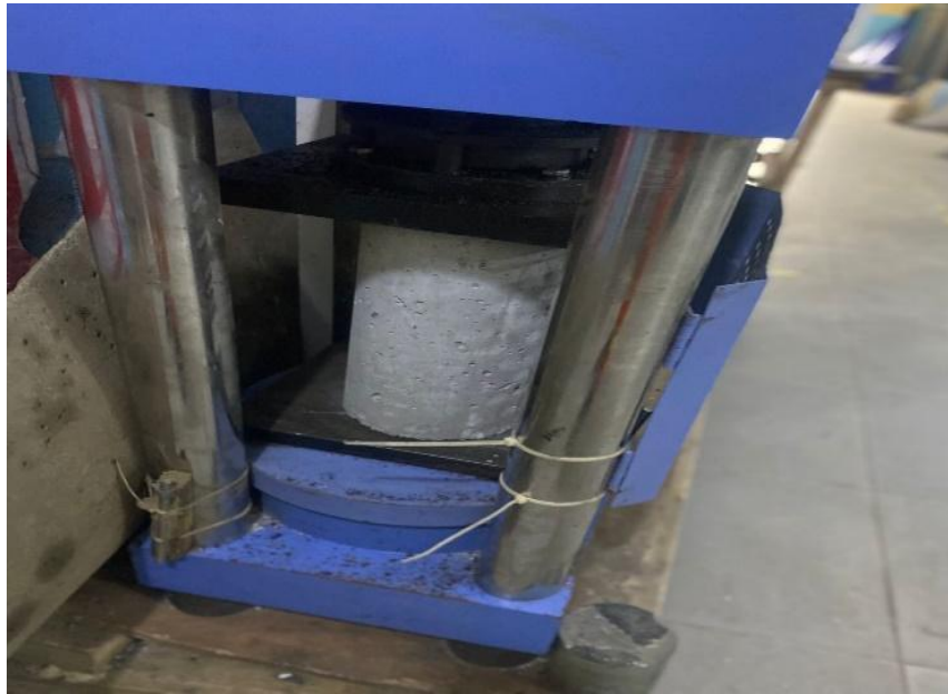
Figure 8: Crushing of test samples at 28 days
