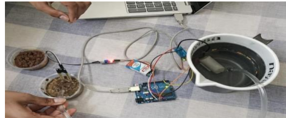
Fig. 2. Experimental setup showing irrigation operation under a dry-soil condition.
