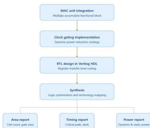
Fig. 1. Workflow of the Proposed Clock-Gated MAC Architecture
