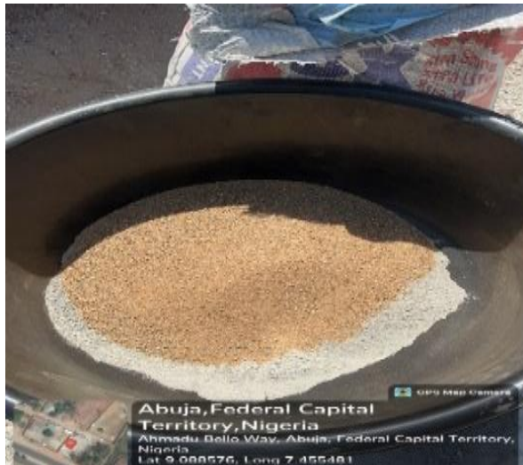
(a) Cement+Fine-Agg.+Laterite+Sawdust Ash
