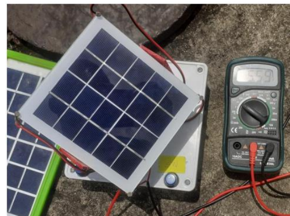
Fig 8: Angle: 150° Voltage: 5.59V 1:21PM
