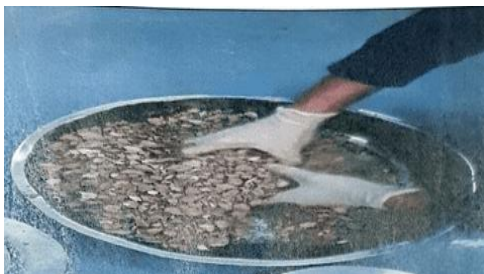
Figure 5 Sample Preparation: Sift the soil sample through a 19 mm sieve, then take 5 kg of the sample and add water to it to obtain the ideal moisture.
