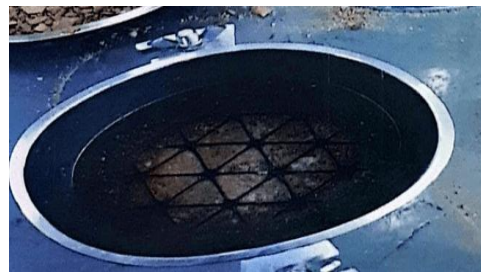
Figure 7 Sample preparation with five-layer compaction using 56 blows per layer and leveling after collar removal.
