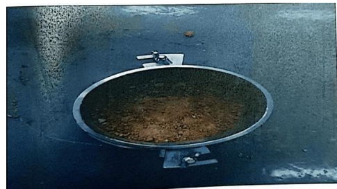
Figure 6 Mold cleaning and oiling, placement of separator disc and filter paper, then filling the mold in five equal parts with the soil-water mixture.
