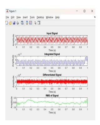
MATLAB for algorithmic development and HDL Coder for subsequent hardware realization. The application of fundamental numerical techniques, specifically the backward difference method for differentiation and rectangular integration for integration, proved to be an efficient approach with a clear pathway to hardware implementation.
