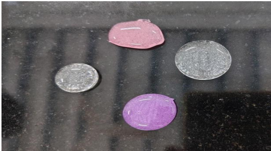
Figure 2. Visual appearance of synthesized phosphate glass samples: undoped, Er 3+ -doped, and Nd 3+ -doped variants.
