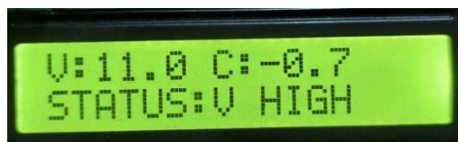
Figure 3: Result of the System when High Voltage
