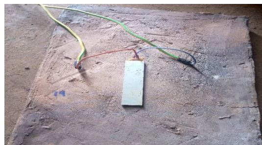
Figure 3.10: Heating the insulating ceramic board with a heating plate
