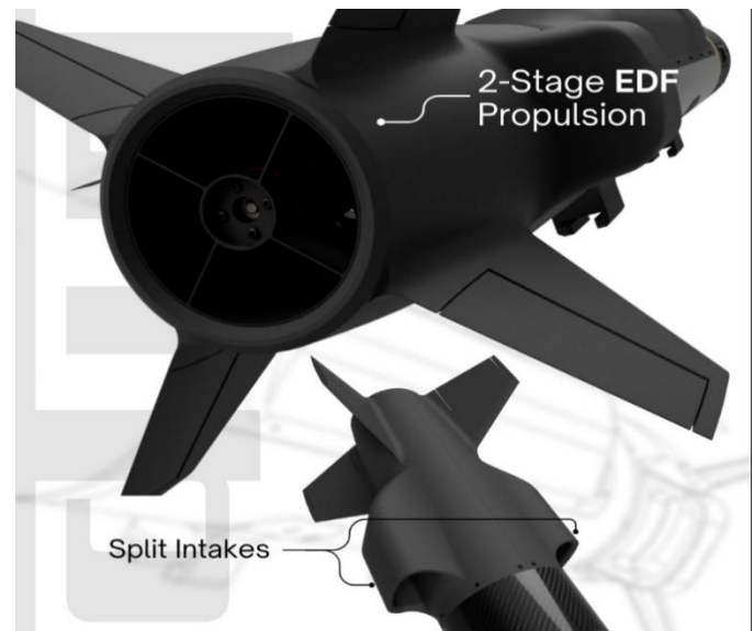
Figure 1: Design of 2 stage EDF Propulsion system integrated in Micro Surface to air missile
