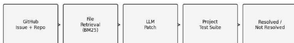
Figure 6: SWE-bench evaluation pipeline (Jimenez et al., ICLR 2024)
