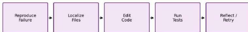
Fig. 4. Agentic program repair workflow (iterative localize–patch–test cycle).
