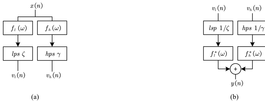
Fig. 2. Block diagram representing a single level TQWT filter bank with: (a) analysis; and (b) synthesis filter bank.
