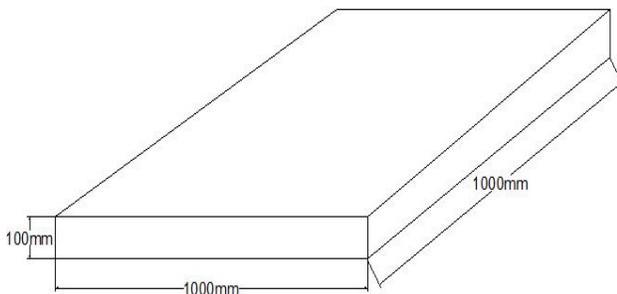
Fig. 1 Geometry of two way slab
