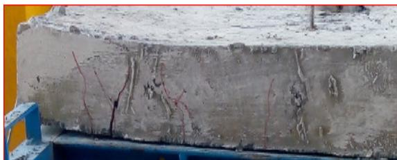
Fig.9 Corner uplift of CON slab
