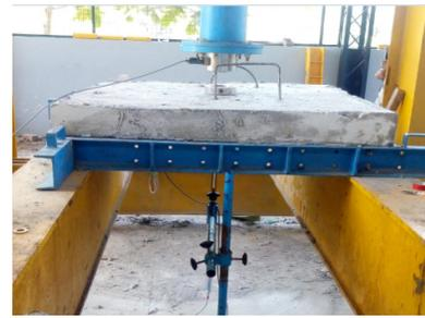
Fig 4 Test setup of specimen
