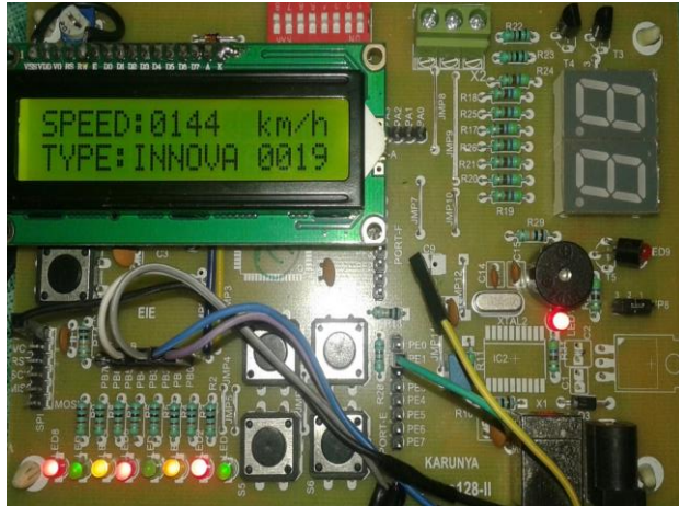
Figure 14: INNOVA Detection and Speed Monitoring
