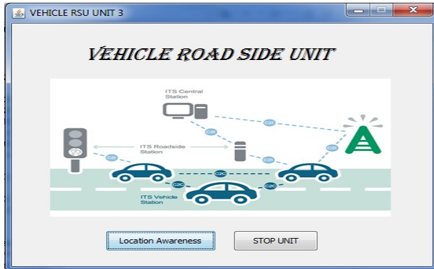
Fig. 13 Press the Location Awareness button to check out the details of the vehicles detected and being forwarded to the other RSU's.
