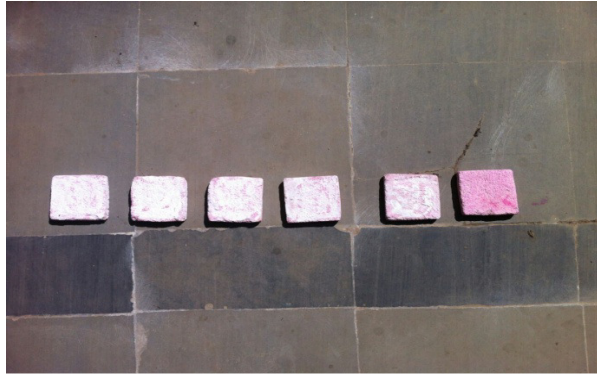
Fig. 3. Visual observation of coated and uncoated surface of TiO 2 sprayed with RhB solution
