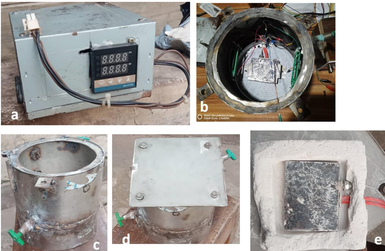
Fig. 1 (a) Temperature control unit, (b) Aerial view of sensing chamber showing the heating plate and connecting wires, (c) Lateral view of the chamber, (d) Closed sensing chamber, and (e) The heating unit.
