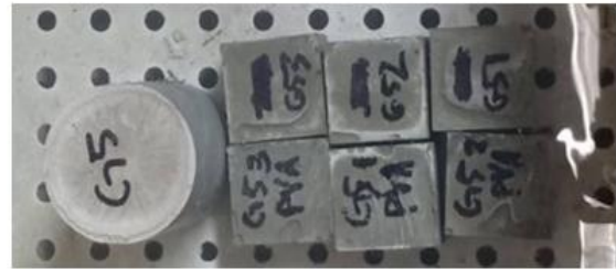
Two days old specimen in the curing tank
