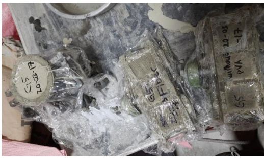
Fresh specimens cast in molds
