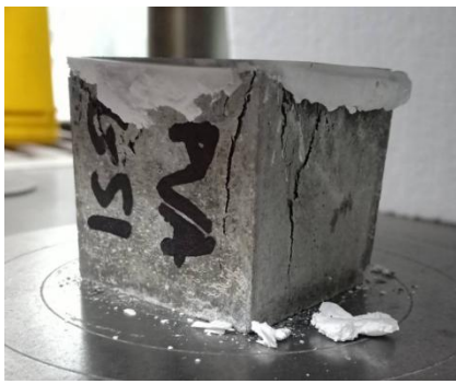
PVA Reinforced Mortar Cube 1
