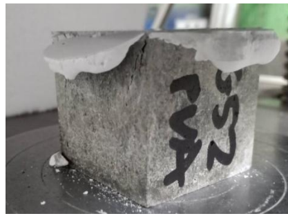
PVA Reinforced Mortar Cube 2
