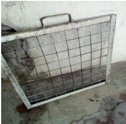
Figure 3.2: Locust bean dryer tray
